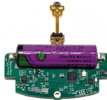
Military sensing system 20Yr life on a single battery
