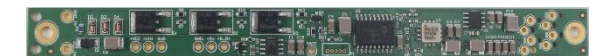
Ultra High temperature (150C+) down oil well precision sensing system (communicates over 5 miles deep)
